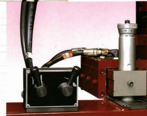
Hydraulic parallel dresser system (must be installed at factory)
